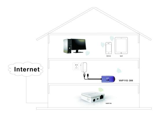
2. Intelligent WiFi Bridge mode(VAP11G-300): WiFi intelligent bridge function, wireless to wired, wired to wireless intelligent switching.
